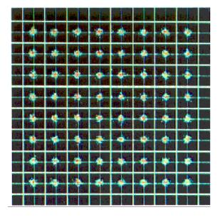
64 QAM signal without faults
